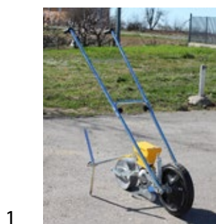
Seminatrice manuale monofila con 5 dischi Single-row manual seeder with 5 aluminum disks
